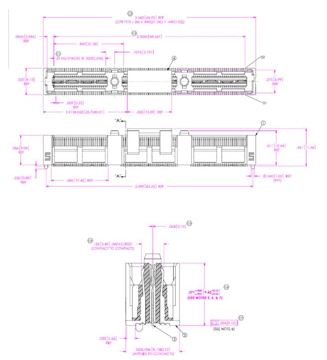
7.1.3. ASP-129646-03 or equivalent (Bottom Connector) Mechanical Drawings
