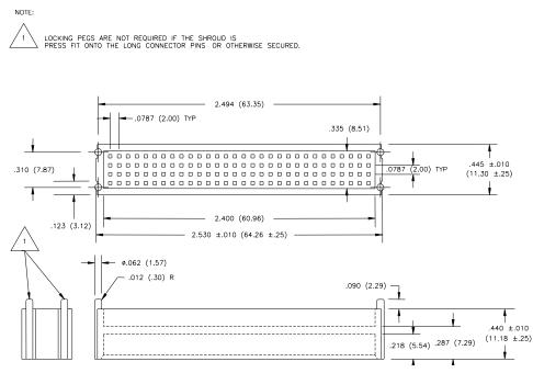
Figure 11 PCI Connector Shroud Mechanical Drawing
