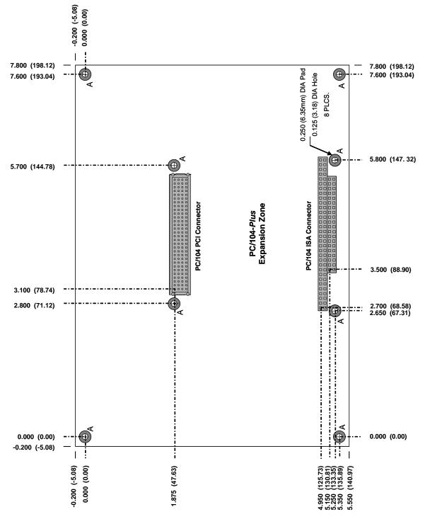
Figure 3 EBX Detailed Mechanical Drawing
