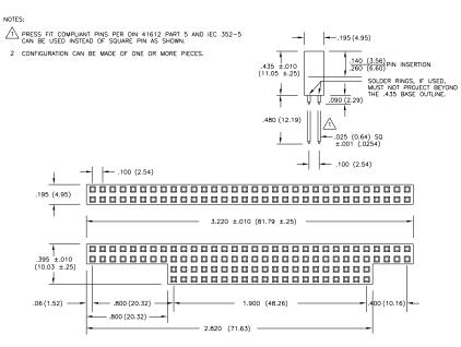
Figure 12 ISA Connector Mechanical Drawing
