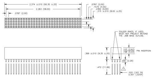
**Figure 10 PCI Connector Mechanical Drawing**
